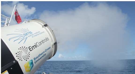
Southern Cross University's MCB sea water spray pump
